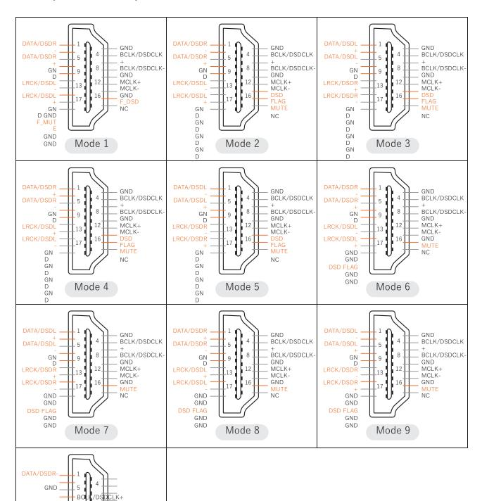
Note: Go to Output settings, switch to IIS output and then tap " "gear icon to set the matching IIs Mode for the DAC.
